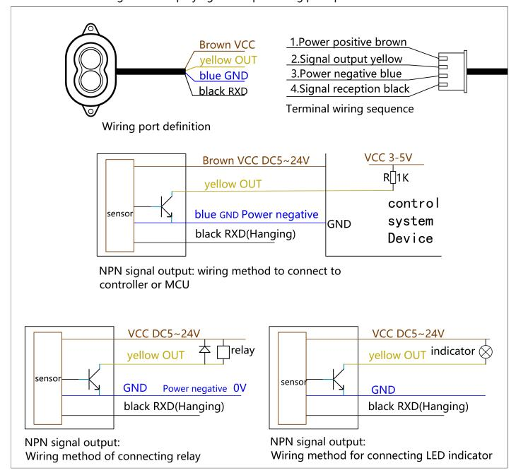
NPN output drive small relay (coil current 300 mA) Operating principle:
