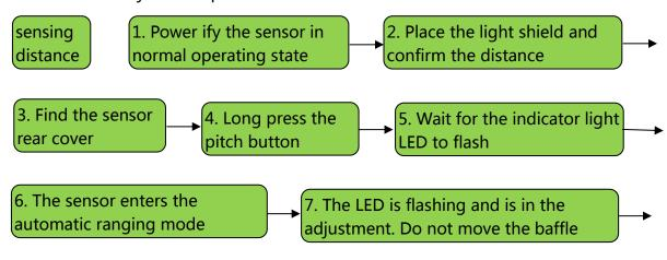
8. The LED indicator light stops flashing, and the distance adjustment is completed.
